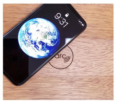
The ARC-H through surface wireless charger offers the ultimate in charging convenience. With a charging range of 15-30mm, ARC-H can be installed without the need to rout into the underside of the surface for surface thicknesses up to 25mm. Once installed ARC-H is completely hidden requiring a simple decal to guide placement of mobiles on the surface.
